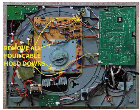
2) Cut the cable hold-downs carefully. Do not cut the wires!
